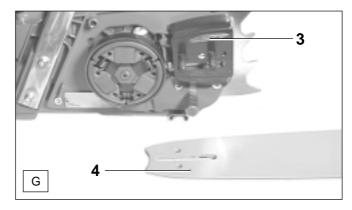
To ensure troublefree operation of the oil pump the oil guide groove at the crank case (G/3) and the oil inlet bore in the guide bar (G/4) must be cleaned regularly.
